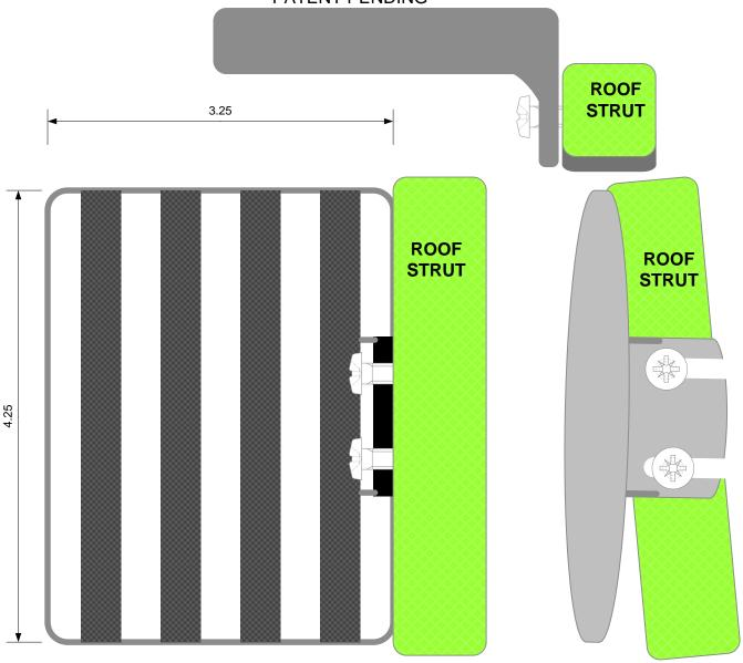
**USE THE WASHER** HEAD SCREWS INCLUDED TO ATTACH THE MIRROR TO THE FORWARD ROOF STRUT
